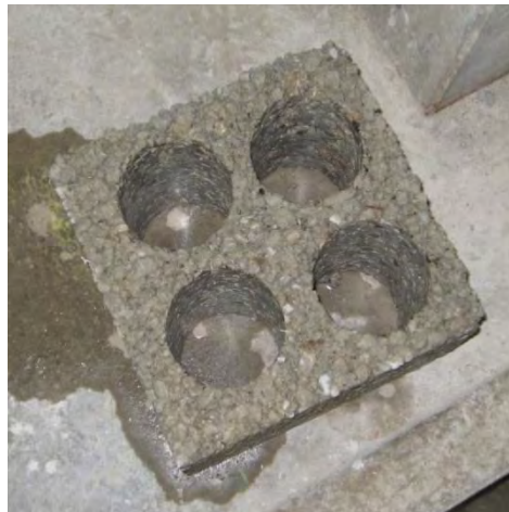
Figure 27. Cores extracted from slabs for material characterization.
