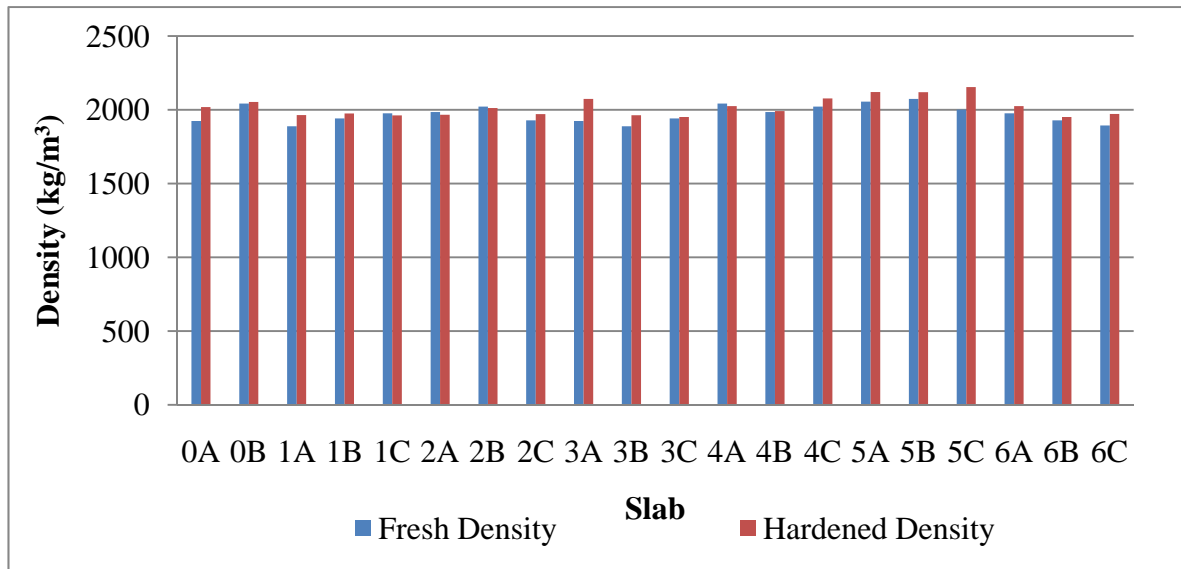
Figure 26. Density of the pervious concrete batches.
