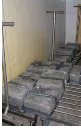
Figure 23. Slabs covered in plastic during curing.
