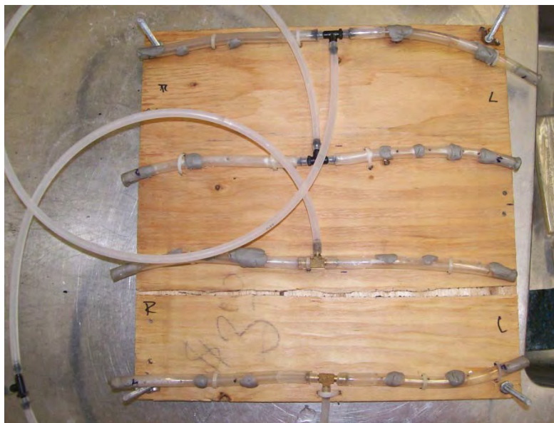
Figure 31. ‘Precipitation’ apparatus used for the application of the water and the brine solution evenly to the surface of the pervious concrete slab
